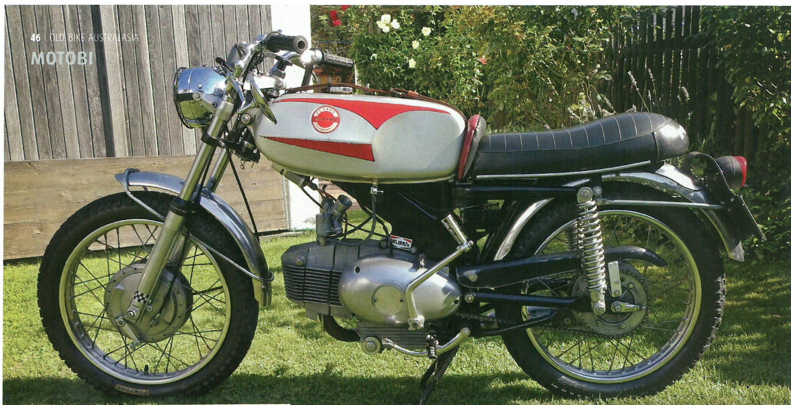
LEFT & ABOVE The 125cc Motobi Sport Special with its Dellorto U822BS carburettor produced 10hp @ 9000rpm, resulting in a top speed of 120km/h.
