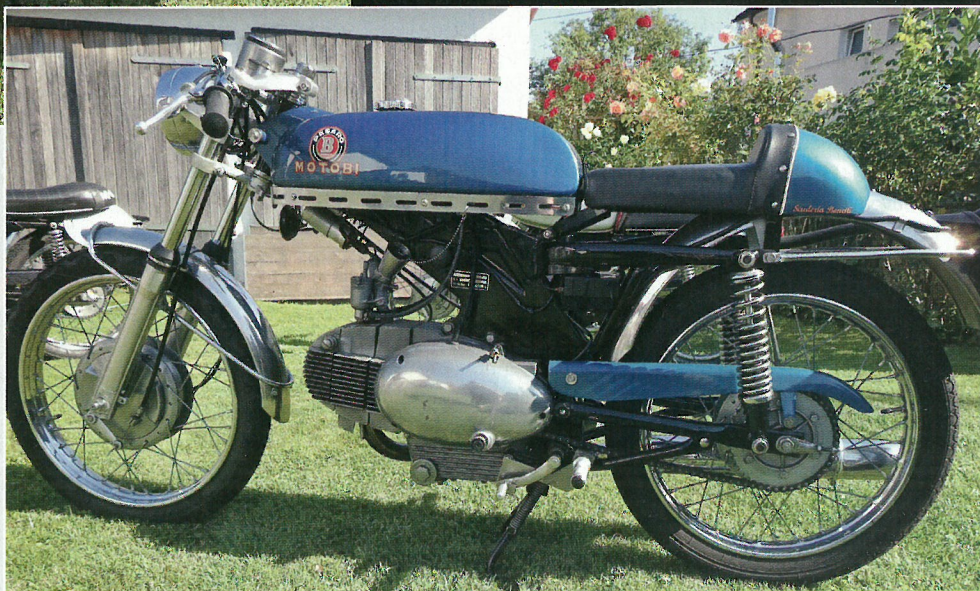
TOP & ABOVE The 250 1970 Motobi (Benelli badged) had a power output of 16.5hp, which netted it a top speed of 140km/h. LEFT & BELOW Motobis are lightweight machines. This 1970 250 Motobi with its Silentium mufflers tops the scale at 102kgs.
