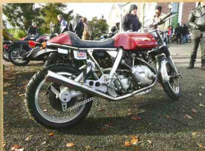
Left: Lovely flowing lines of Snowdon's 1935 Indian Chief sidecar rig. Right: Here's something you don't often see: a custom Vincent built by UK expat Chris Kibbs that uses a spine-type aluminum frame based on the geometry of a Ducati 900SS.
